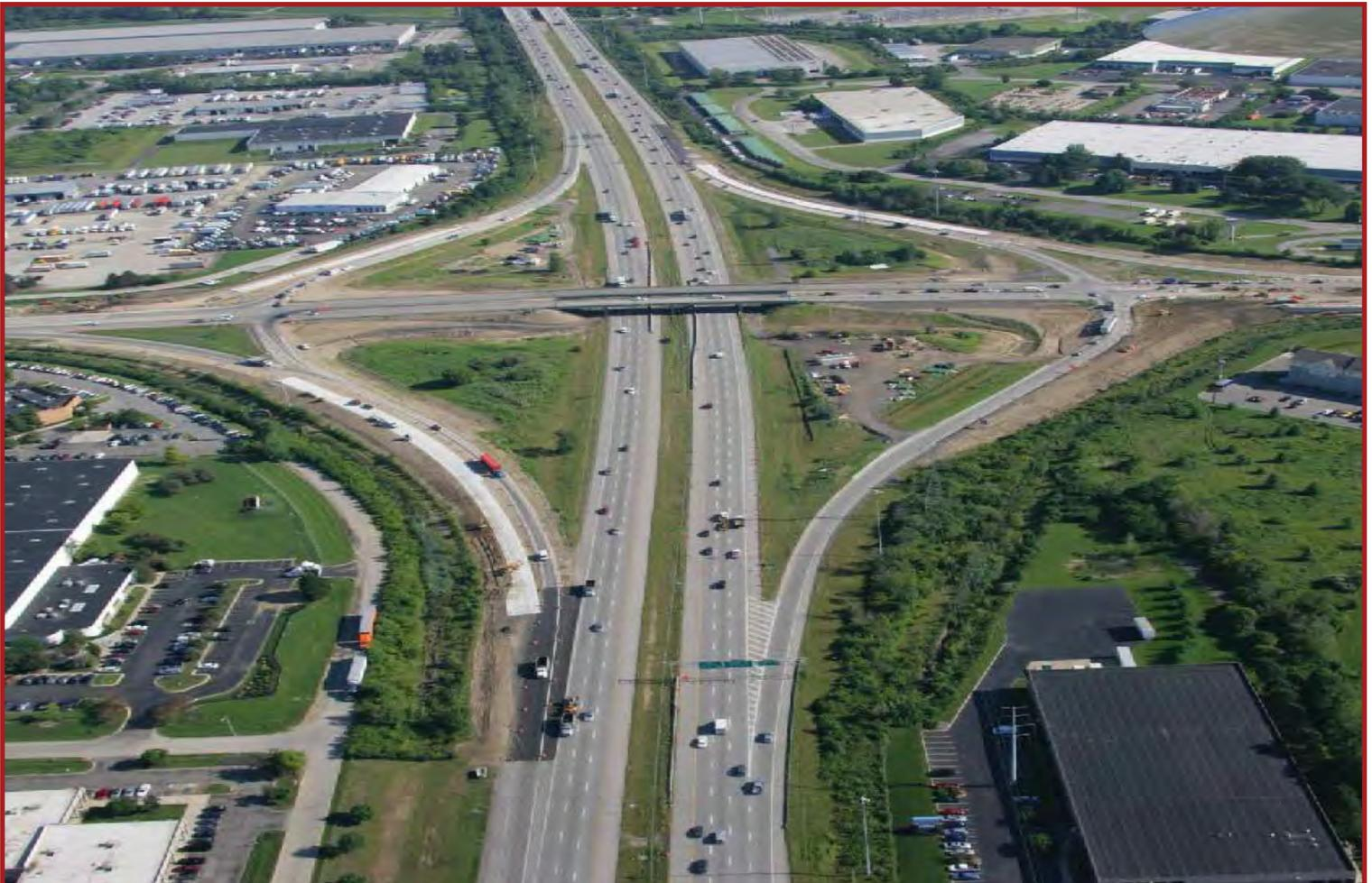
the nodes of the interchange. Once there, vehicles can turn left onto freeway ramps to enter the highway (I-270) without stopping or conflicting with opposing through traffic. By eliminating left turns that cross opposing traffic like those at conventional intersections, the number of potential conflict points is reduced by 42 percent compared to a traditional diamond interchange. The number of crossing conflict points, typically resulting in the most severe crashes, is reduced by 80 percent.
